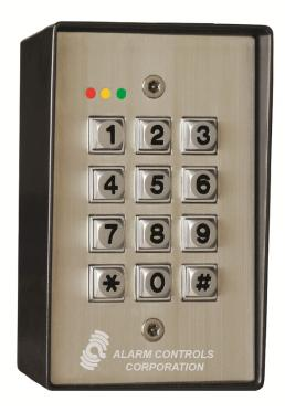
Model KP-400 is a self-contained vandal resistant digital keypad. This dual-relay output keypad is suitable for residential, industrial, and commercial installations. It is compatible with all electric locking devices. Durable backlit metal keys and a rugged metal housing protect the keypad from harsh environments.
