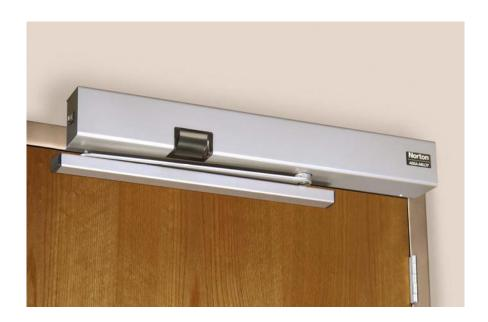
The Norton 7100SZ style door closer combines with a manifold and solenoid to provide a hold-open feature. When the door is opening manually, SafeZone® senses movement in the door opening and stops the door from closing.
