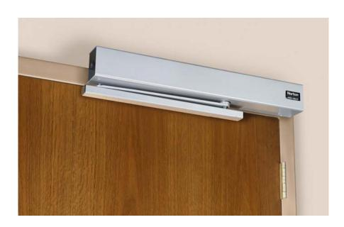
Use a Norton 7200 style door closer combined with a manifold and solenoid to provide a hold-open feature. When the door is opened manually beyond an adjustable hold-open point and released, the solenoid is energized and the door will remain open.
