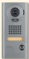
IS-IPDV IP Video Door Station • PoE or 24V DC • PTZ camera • Aluminum die cast cover • Weather and vandal resistant • Surface mount
