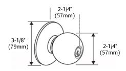
Knob projections shown are for 1-3/4" (44mm) thick doors and will vary by door thickness.
