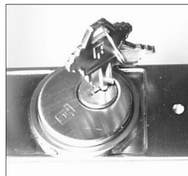
Fig. 1a: Insert key 1/2 way into cylinder and screw in
