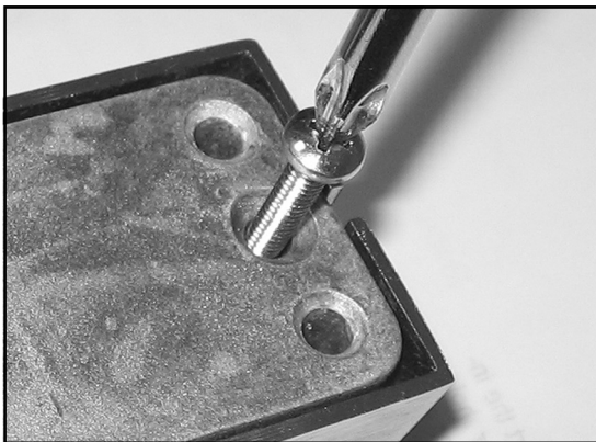
Fig. 7: The Phillips screw on the rear side locks or unlocks the battery cover. Do not remove screw.
