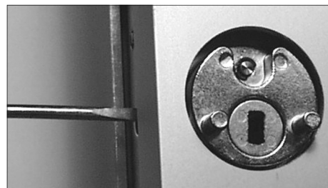
Fig. 5d: Tighten the interface cylinder set screw
