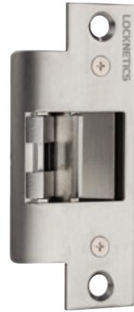
The no cut electric door strike can be used to convert cylindrical lock sets into an electronic access controlled locking system. No cutting on the frame is required. Simply adjust the vertical alignment feature to the latch bolt centerline and install.
