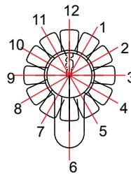
Multi-indexing cam with 12 positions. Cam is set at 5 o'clock from the factory
